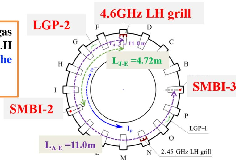
The fastest feedback response time is SMBI fed on the electron-drift side and the slowest response is LGP, between which is SMBI fed on the ion-drift side.
