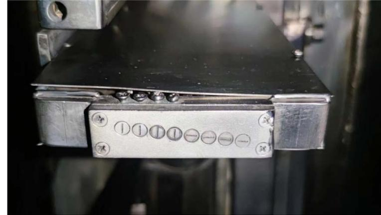
Probe array installed near LH antenna
