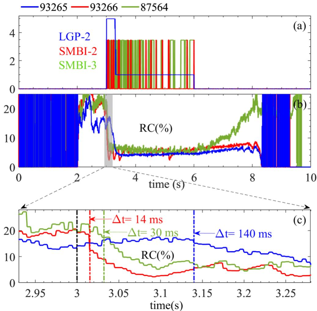
1. LGP-2 vs SMBI-2, located in the electron-drift side of the LH antenna  $\Rightarrow$  SMBI-2 is better than LGP-2, mainly due to different response time of fueling system.
