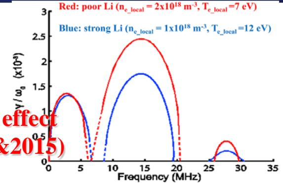
**PDI (Parametric Decay Instability)** is one of important candidates for the **Decrease of LHCD efficiency at high density**. Improving CD capability by **reducing recycling** or **improving LH source frequency** is documented in EAST.
