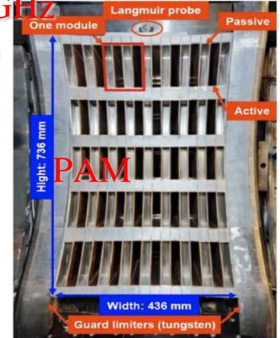
20 main waveguides arranged in an array of 5 rows and 4 columns. (20 klystrons)
