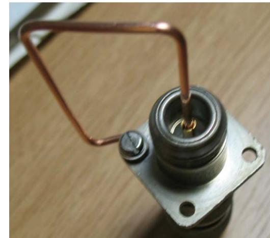
Loop antenna for frequency spectrum
