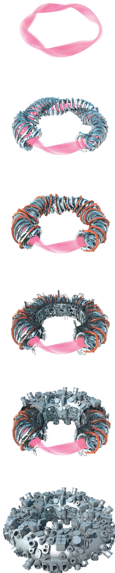
Stellarator Wendelstein 7-X: The graphics show from top to bottom the plasma shape, the superconducting stellarator magnet coils, the planar magnet coils, wiring, cooling lines and inner support structure, parts of the outer vessel and the entire outer vessel. (Graphic: MPI for Plasma Physics)
