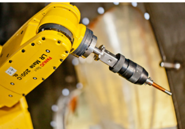
Robots used to position roughly 6,000 bolts and mountings to the inside wall of the plasma vessel.
