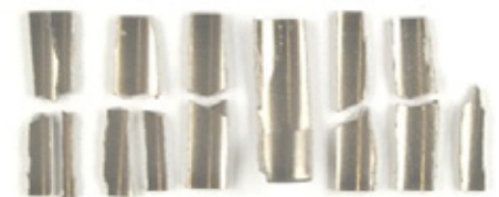
Fractures in brittle, solid tungsten and the ductile behaviour of laminated tungsten notched-bar impact testing
