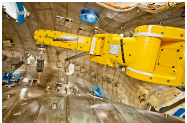
Robots used to position roughly 6,000 bolts and mountings to the inside wall of the plasma vessel.
