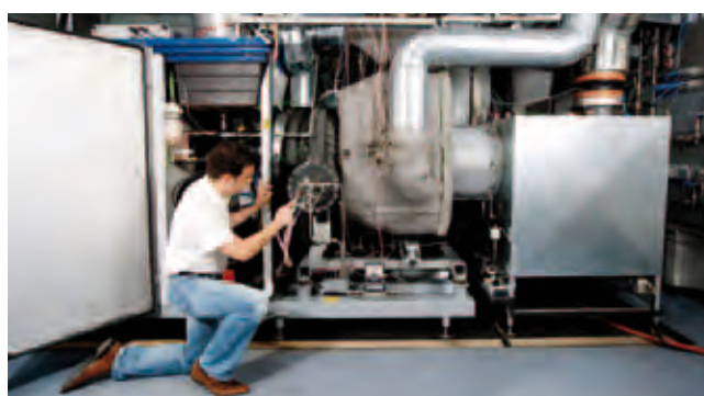
Test stand for optimising a micro gas turbine.
