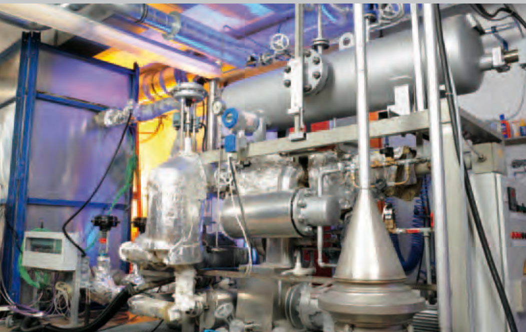
Test facility for high-temperature heat stores using salt media (left).
