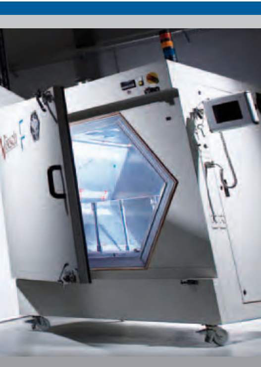
HEPHAISTOS, the world's biggest microwave processing plant (left). Karlsruhe Institute of Technology
