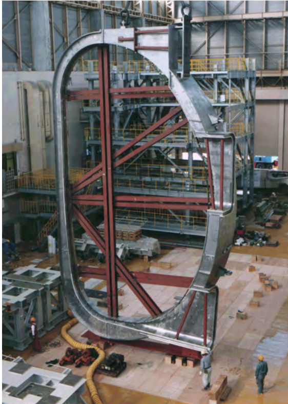
Full-size prototype of sector of the ITER plasma vessel, built in Japan according to the ITER design of 1998
